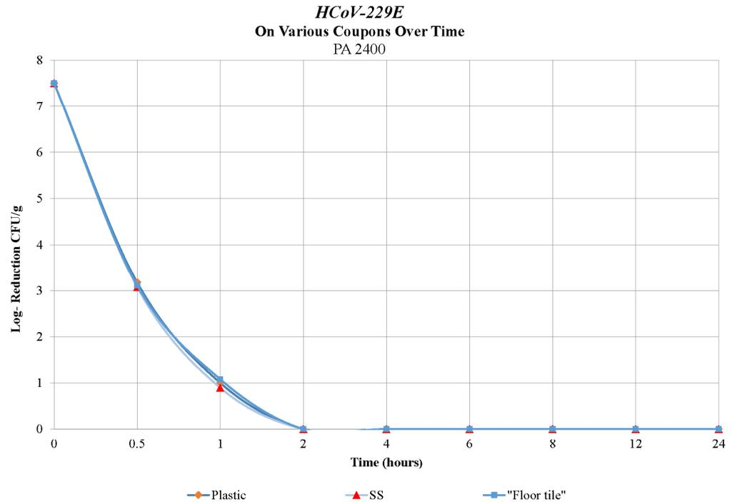
\* Tests conducted by Scientific Air Solutions, a Biosafety Level 2 facility, in a test chamber (6' x 4' x 10') by exposing coupons inoculated with indicated organism – reflects actual virus and reductions over time. Advanced oxidation system developed by airPHX company.
